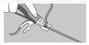
• With a trimming plane: rotate the trimming guide to 90° on the side. Trim the weld after it has cooled down. Tools available from Janser or Romus.
